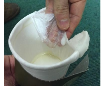
Picture 1: After soaking the single use cup which looked papery... one can rub off the paper and see the plastic.
